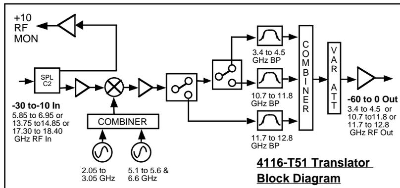
**FIGURE 1. Model 4116-T51 Multi-Band Block Translator Block Diagram**
