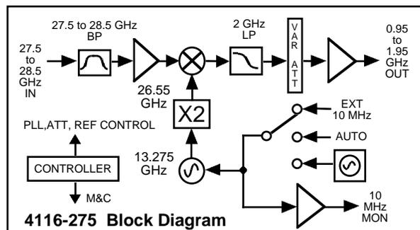
FIGURE 1. Model 4116-275 Ka-Band Block Downconverter Block Diagram
