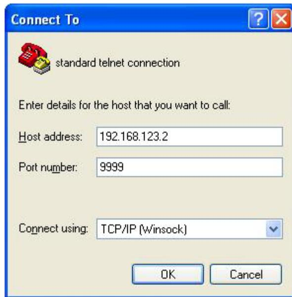
**Figure 2-E: - Telnet® Settings in Hyper Terminal**
