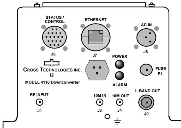
Model 4116-275 Ka-Band Block Downconverter, Front Panel
