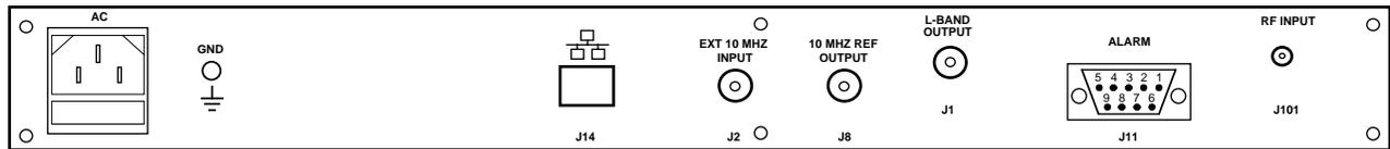
REAR PANEL - 3116-277#-1200 (Shown with optional RJ45 Ethernet Connector)
