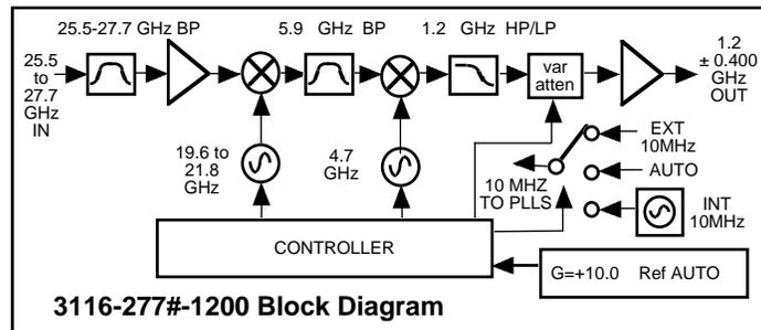
FIGURE 1.2 3116-277#-1200 Block Diagram
