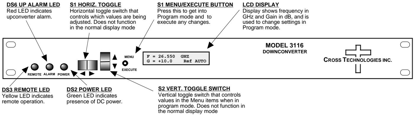
**FIGURE 2.2 3116-277#-1200 Front Panel Controls and Indicators**
