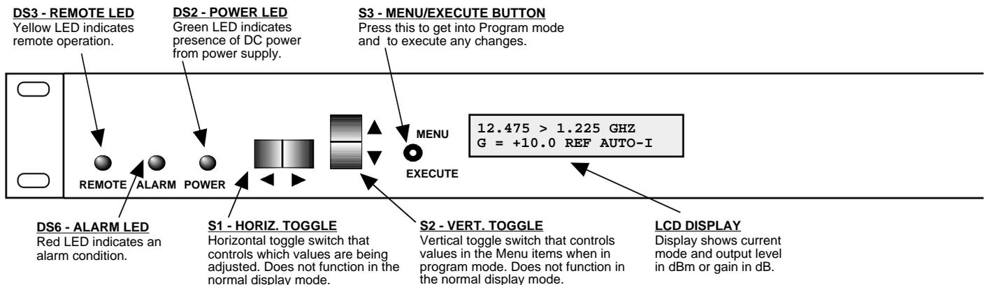
FIGURE 2.2 3116-125 Front Panel Controls and Indicators
