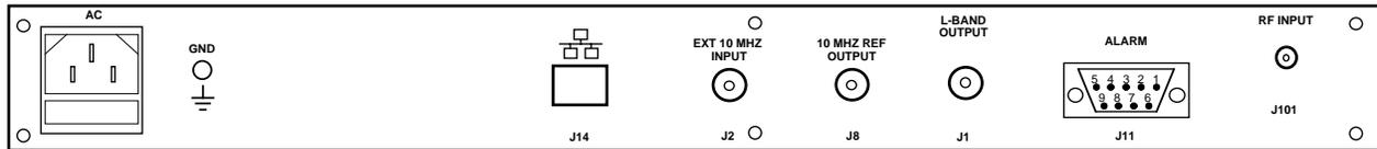
REAR PANEL - 3116-125 (Shown with optional RJ45 Ethernet Connector)
