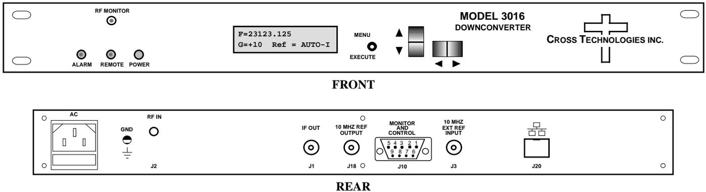
**FIGURE 1.1 Model 3016-2124 Front and Rear Panels**
