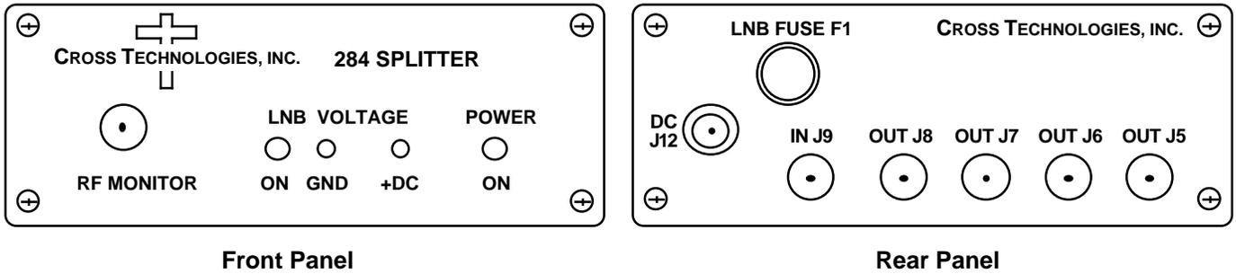
**FIGURE 1.1 MODEL 284-15 Front and Rear Panels**
