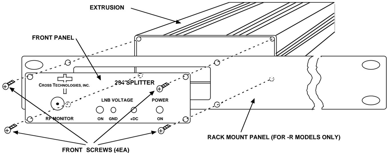
**FIGURE 2.5** Rack Mounting the 284-09
