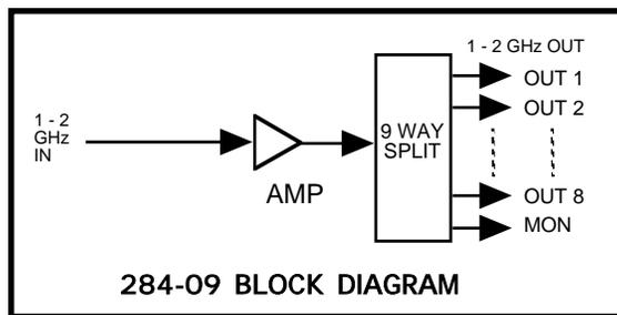
**FIGURE 1.3 Model 284-09 RF Splitter Block Diagram**
