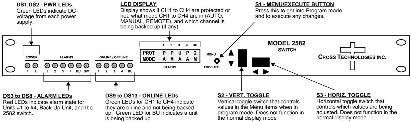
**FIGURE 2.2 2582-144 Front Panel Controls and Indicators**
