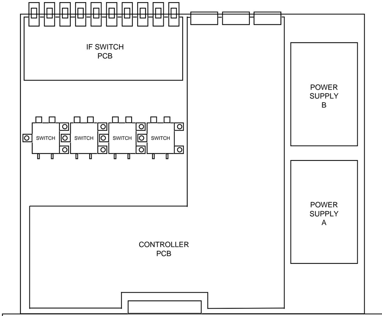
**FIGURE 2.0 2582-144 Mechanical Assembly**
