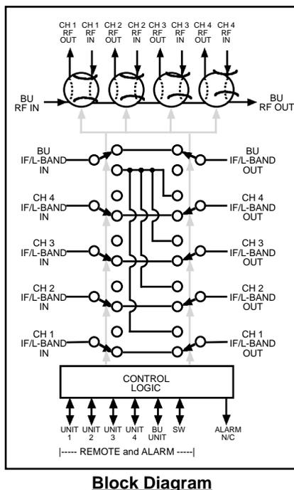
**FIGURE 1.2 Model 2582-144 Switch Block Diagram**
