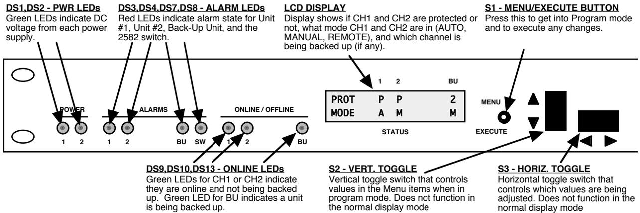
**FIGURE 2.2 2582-122 Front Panel Controls and Indicators**
