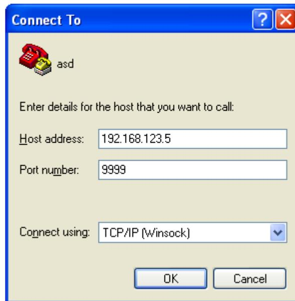
**Figure 3.4: Telnet<sup>®</sup> Settings in Hyper Terminal**
