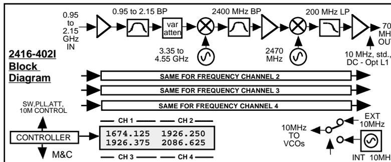
**FIGURE 1.2 Model 2416-x02I Downconverter Block Diagram**
