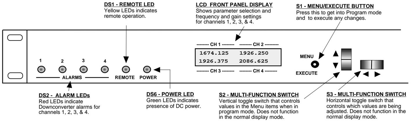
**FIGURE 2.3 2416-x02I Front Panel Controls and Indicators**
