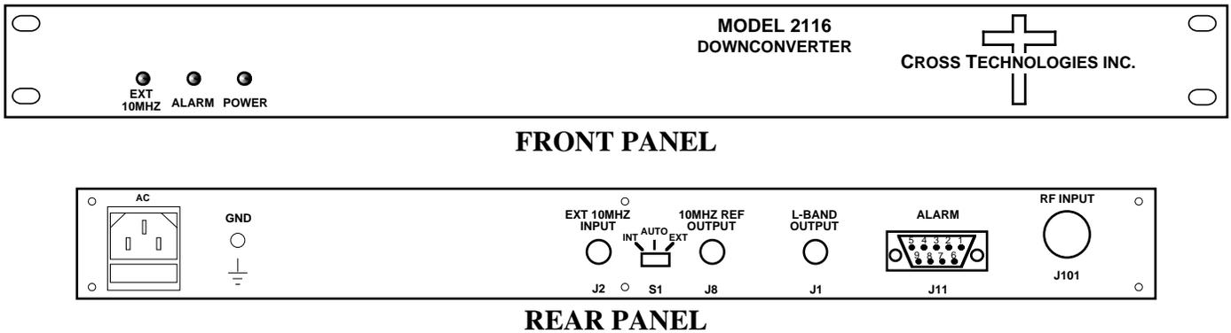
FIGURE 1.1 Model 2116-78#-1100 Front and Rear Panels
