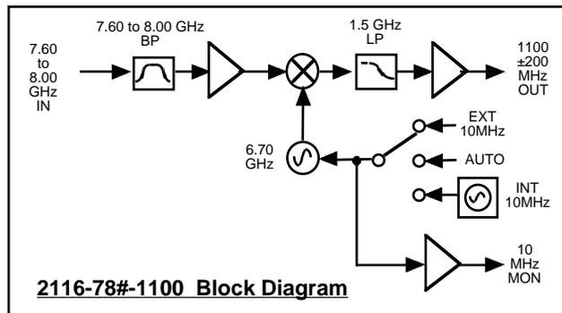
FIGURE 1.2 Model 2116-78#-1100 Downconverter Block Diagram
