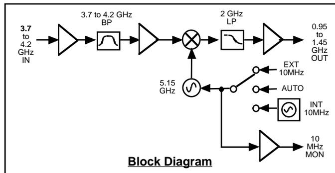
FIGURE 1.2 Model 2116-37 Downconverter Block Diagram
