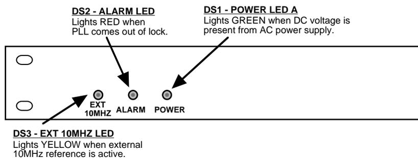
**FIGURE 2.2 2116-310T212 Front Panel Controls and Indicators**
