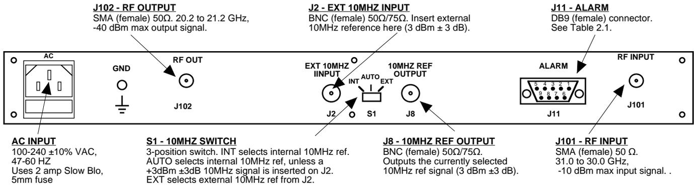
**FIGURE 2.1 2116-310T212 Rear Panel I/O's**
