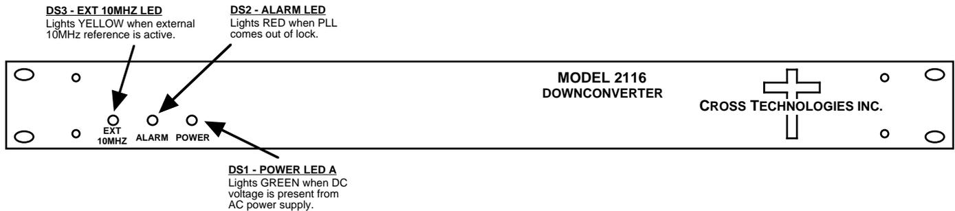
**FIGURE 2.2 2116-275-1800 Front Panel Controls and Indicators**
