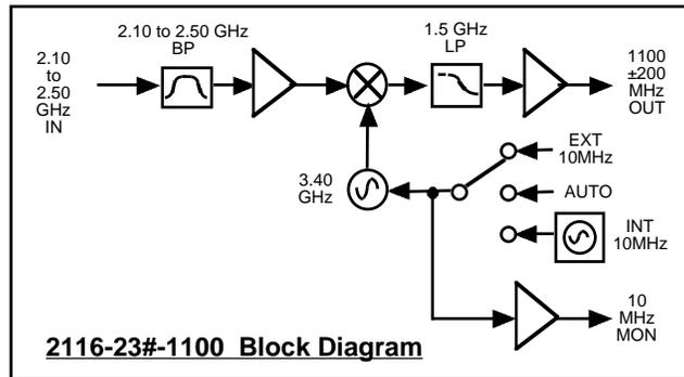
FIGURE 1.2 Model 2116-23#-1100 Downconverter Block Diagram
