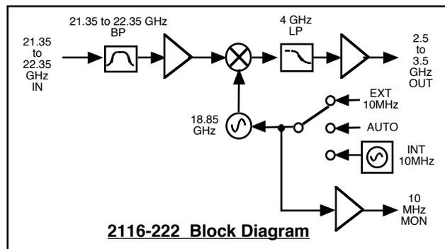
FIGURE 1.2 Model 2116-222 Downconverter Block Diagram
