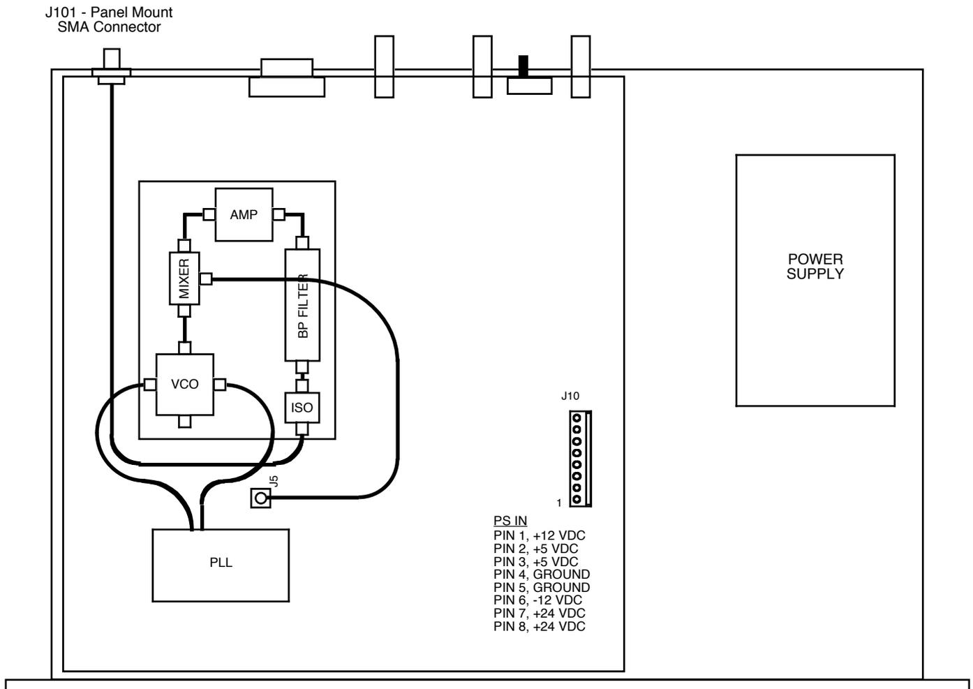
**FIGURE 2.0 2116-222 Mechanical Assembly**
