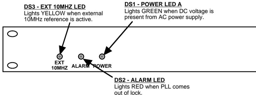
**FIGURE 2.2 2116-14T12 Front Panel Controls and Indicators**
