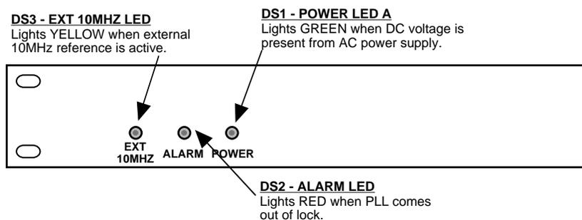
**FIGURE 2.2 2116-13T11 Front Panel Controls and Indicators**
