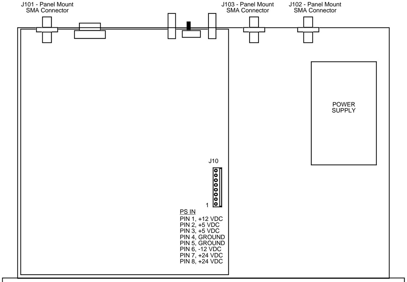
**FIGURE 2.0 2116-13T11 Mechanical Assembly**
