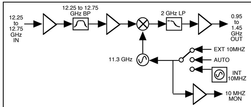
**FIGURE 1.2 Model 2116-126 Downconverter Block Diagram**
