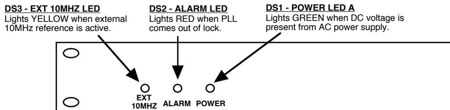
**FIGURE 2.2 2116-114 Front Panel Controls and Indicators**
