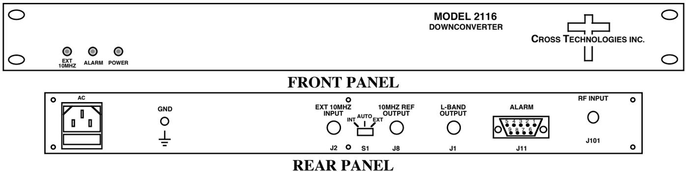
**FIGURE 1.1 Model 2116-114 Front and Rear Panels**
