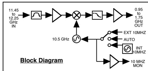
**FIGURE 1.2 Model 2116-114 Downconverter Block Diagram**
