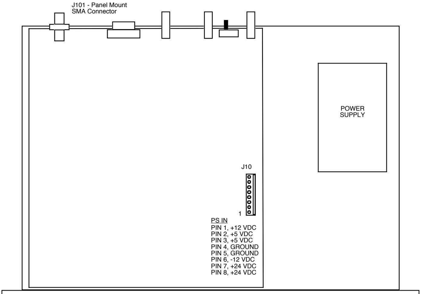
**FIGURE 2.0 2116-107 Mechanical Assembly**
