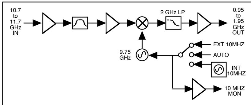
**FIGURE 1.2 Model 2116-107 Downconverter Block Diagram**
