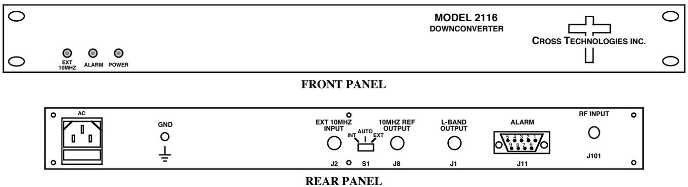
**FIGURE 1.1 Model 2116-107 Front and Rear Panels**
