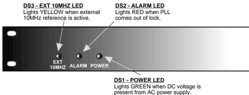
**FIGURE 2.2 Front Panel Controls and Indicators**
