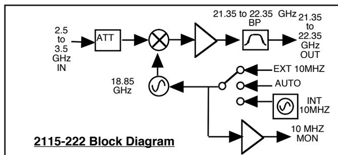
FIGURE 1.2 Model 2115-222 Upconverter Block Diagram
