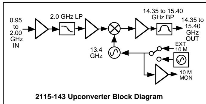
FIGURE 1.2 Model 2115-143 Upconverter Block Diagram
