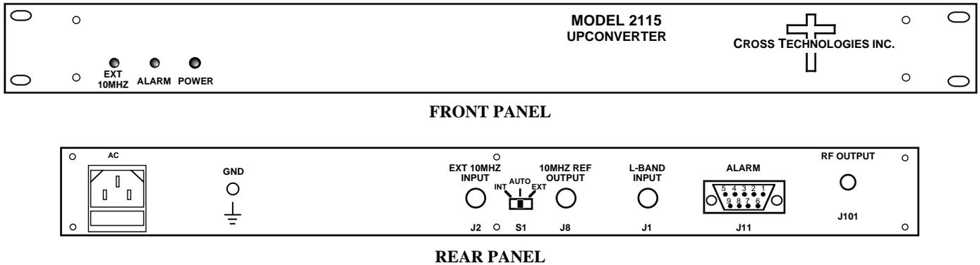
FIGURE 1.1 Model 2115-143 Front and Rear Panels
