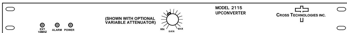
FRONT PANEL - (Shown with Variable Attenuator Option -VA)
