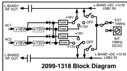
**FIGURE 1.2 Model 2099-1318 10MHz Source/Inserter Block Diagram**
