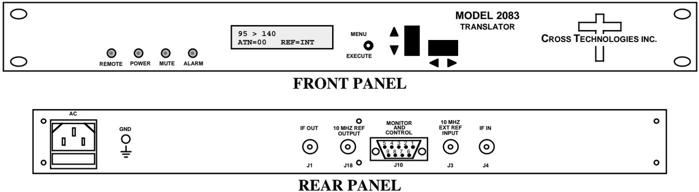
FIGURE 1.1 Model 2083-914A Front and Rear Panels
