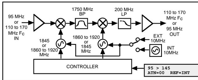
FIGURE 1.2 Model 2083-914A Translator Block Diagram
