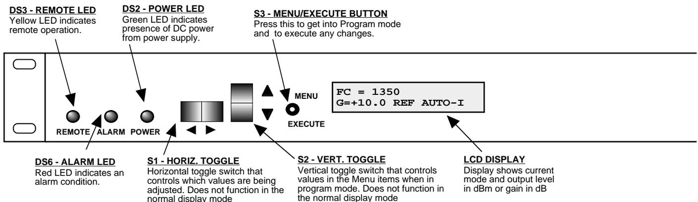
**FIGURE 2.2** 2083-1919-02 Front Panel Controls and Indicators
