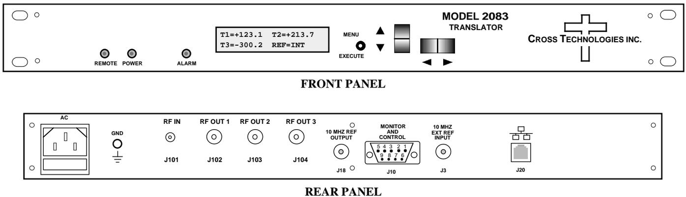
**FIGURE 1.1 2083-13-1518 Front and Rear Panels**
