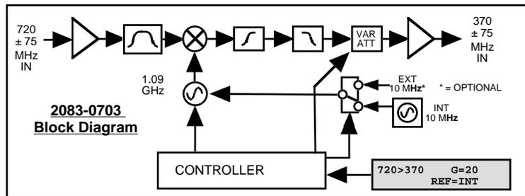
**FIGURE 1.2 Model 2083-0703 Block Diagram**
