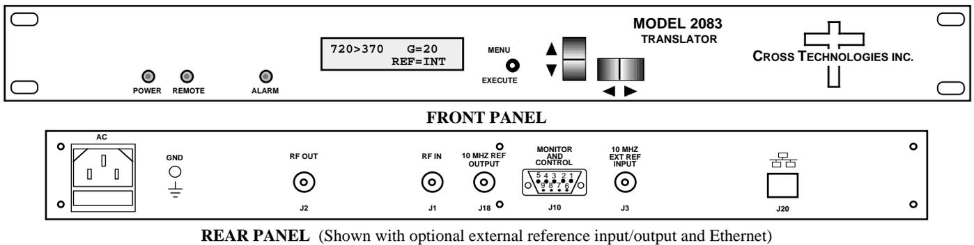
**FIGURE 1.1 Model 2083-0703 Front & Rear Panels**
