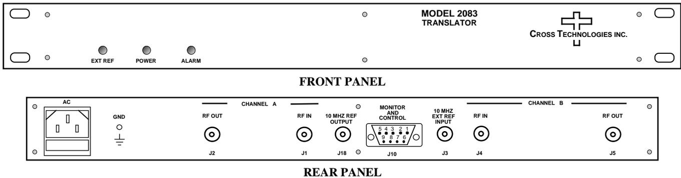
**FIGURE 1.1 Model 2083-0372 Front & Rear Panels**
