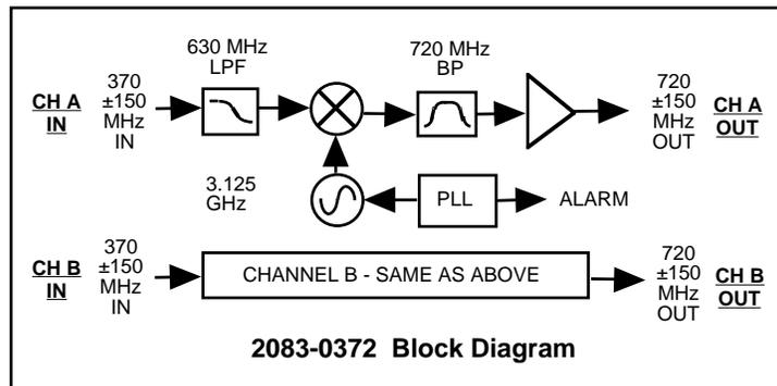
**FIGURE 1.2 Model 2083-0372 Block Diagram**
