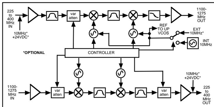
**Figure 1.2 Model 2017-T03-400 Up/Downconverter Block Diagram**
