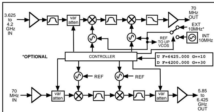
**Figure 1.2 Block Diagram**
