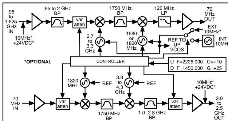
**Figure 1.2 Model 2017-35 Up/Downconverter Block Diagram**
