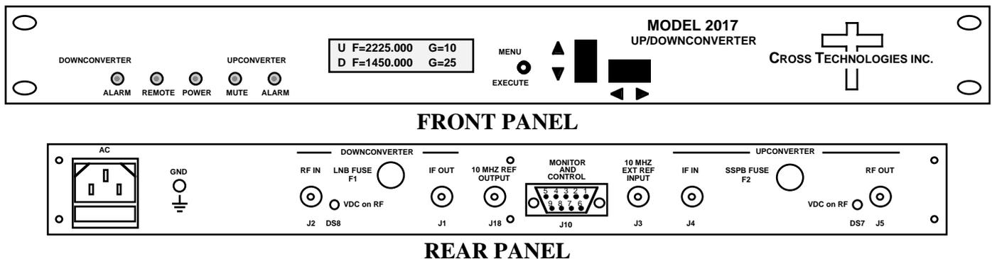
**Figure 1.1 Model 2017-35 Front and Rear Panels**
