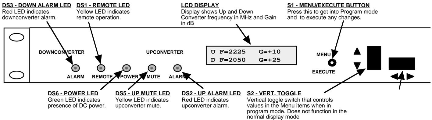
**Figure 2.2 Model 2017-25 Front Panel Controls and Indicators**
