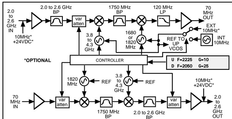
**Figure 1.2 Model 2017-25-02 Up/Downconverter Block Diagram**
