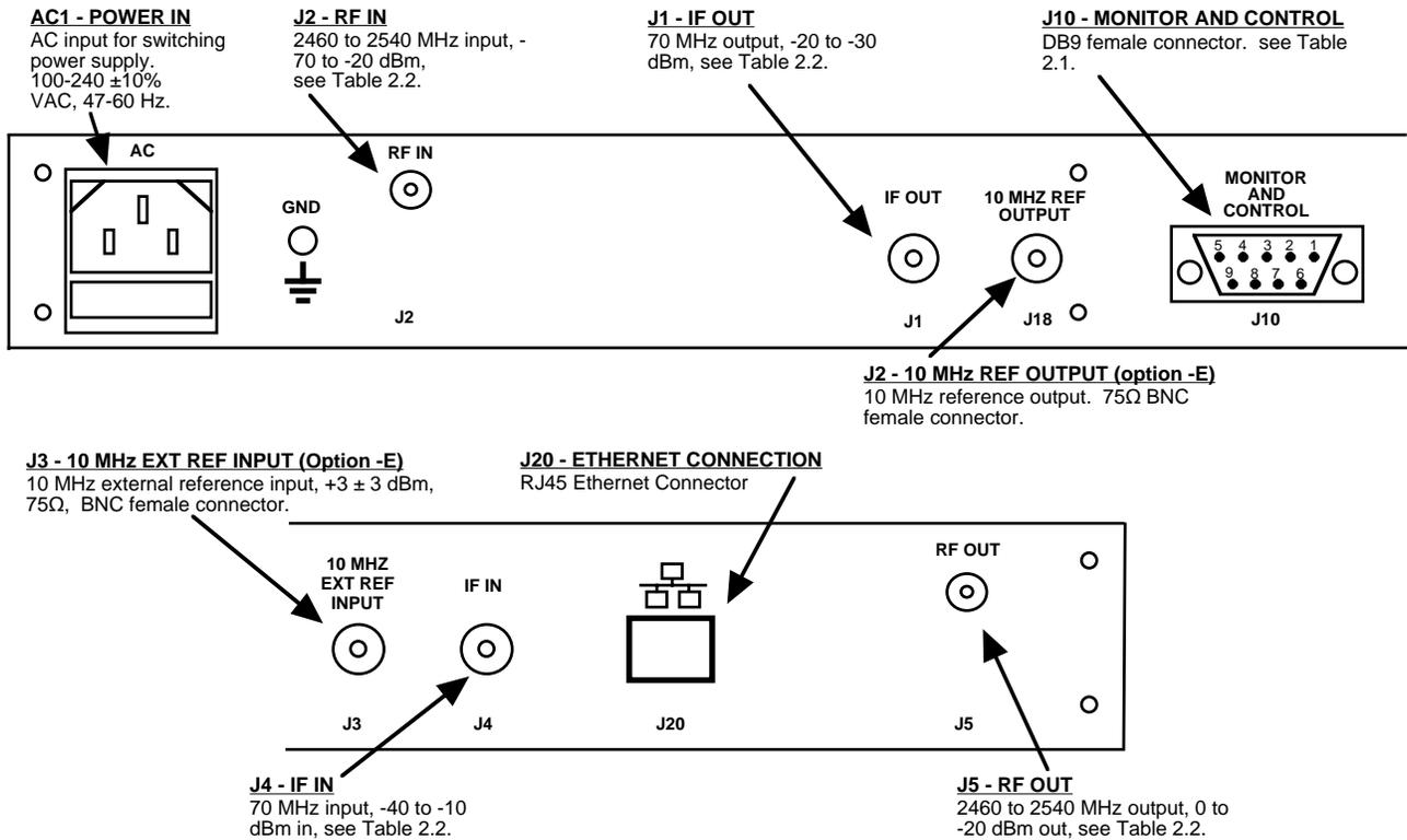
**Figure 2.1 Model 2017-25-01 Rear Panel I/O's**
