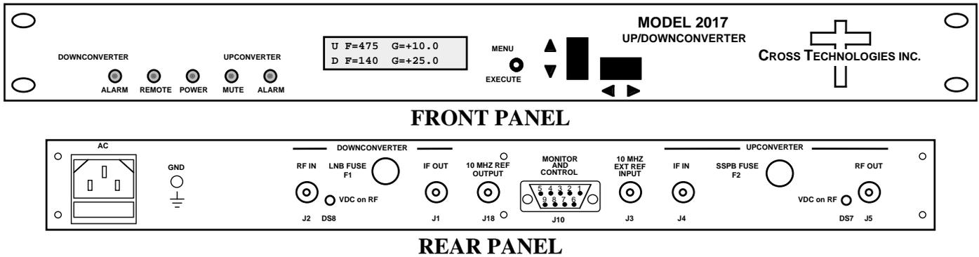
**Figure 1.1 Model 2017-1351 Front and Rear Panels**
