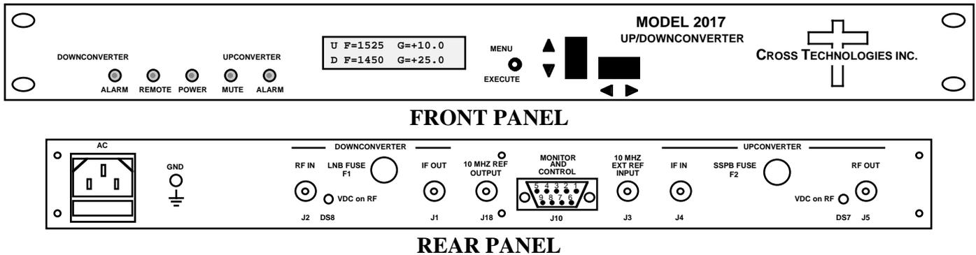
**Figure 1.1 Model 2017-05A Front and Rear Panels**
