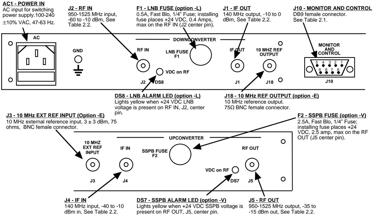
**Figure 2.1 Model 2017-05A Rear Panel I/O's**
