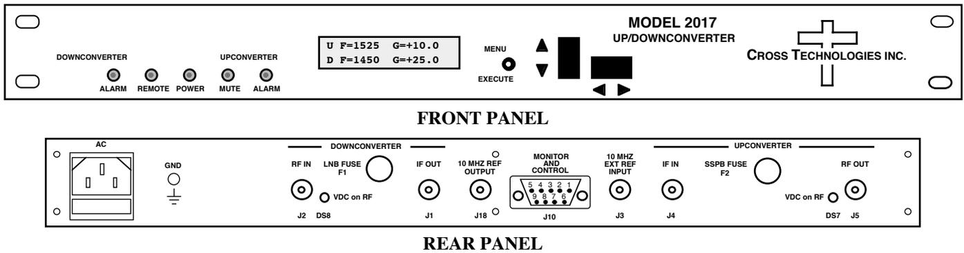
**Figure 1.1 Model 2017-04 Front and Rear Panels**
