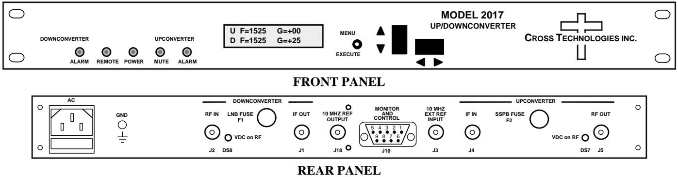
**Figure 1.1 Model 2017-03A Front and Rear Panels**
