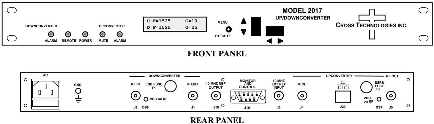
Figure 1.1 Model 2017-02 Front and Rear Panels
