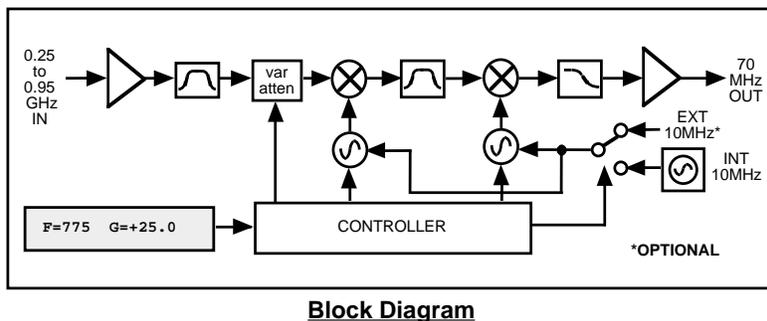
**FIGURE 1.2 Model 2016-95 Downconverter Block Diagram**
