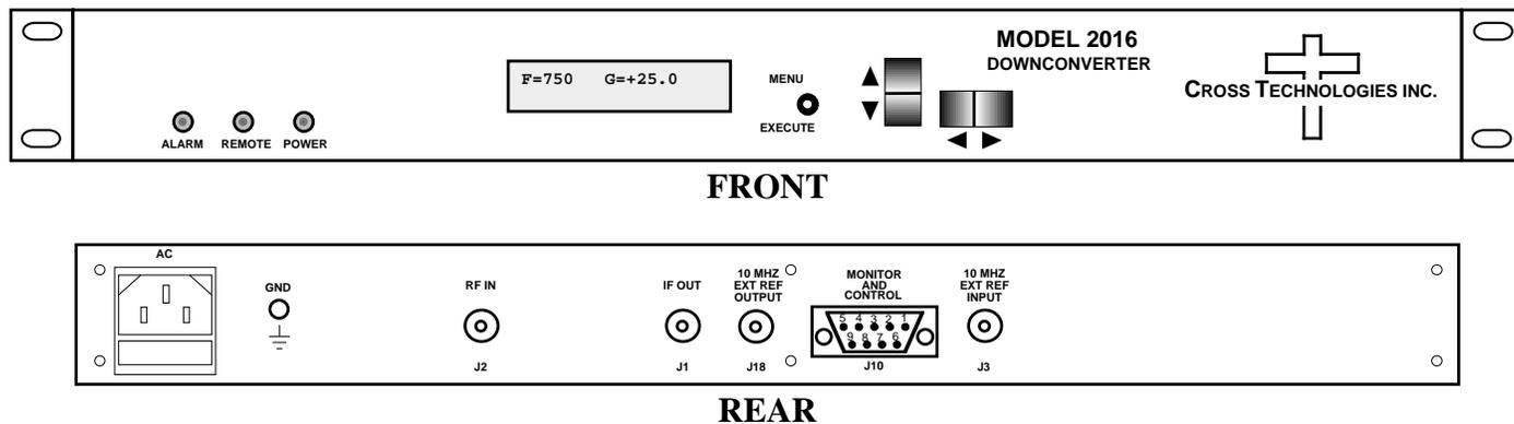
**FIGURE 1.1 Model 2016-95 Front and Rear Panels**
