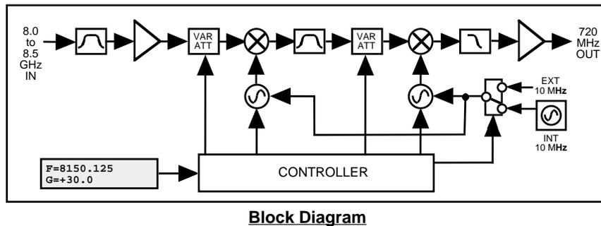
FIGURE 1.2 Model 2016-8085-720 Downconverter Block Diagram
