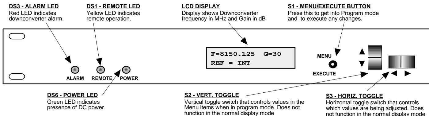
**FIGURE 2.3 2016-8085-720 Front Panel Controls and Indicators**
