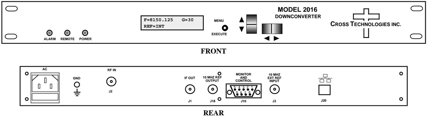
FIGURE 1.1 Model 2016-8085-720 Front and Rear Panels
