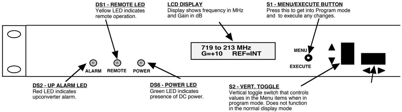
**FIGURE 2.2 2016-75-213 Front Panel Controls and Indicators**
