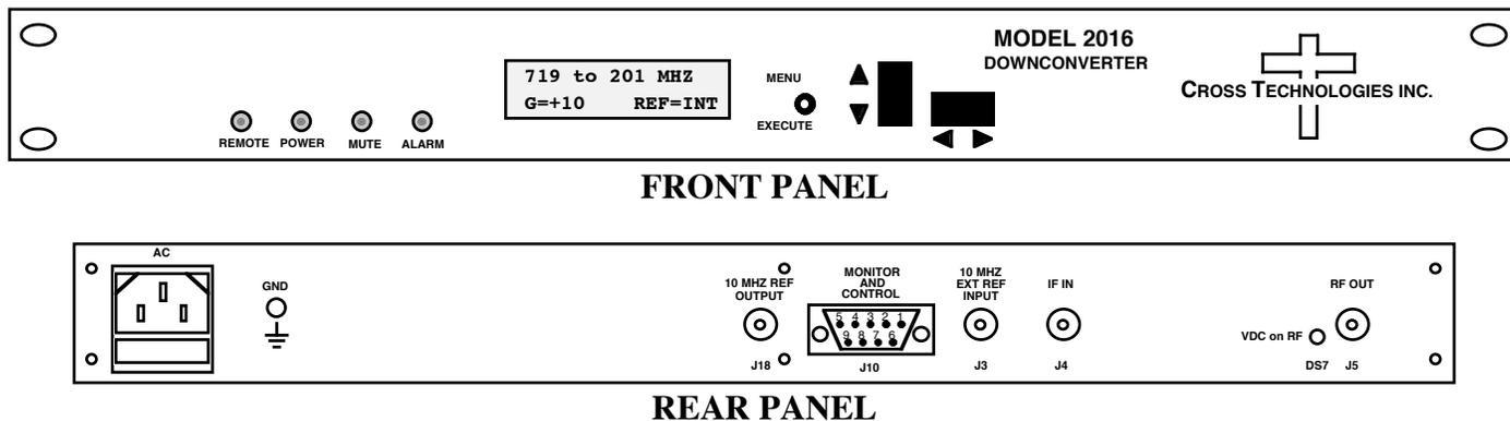
**FIGURE 1.1 Model 2016-75-213 Front and Rear Panels**
