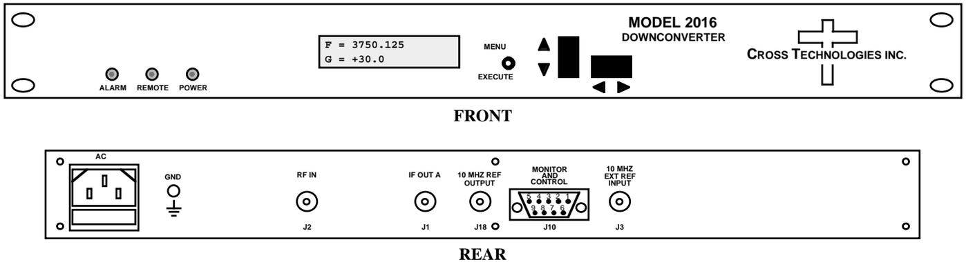
**FIGURE 1.1 Model 2016-37 Front and Rear Panels**
