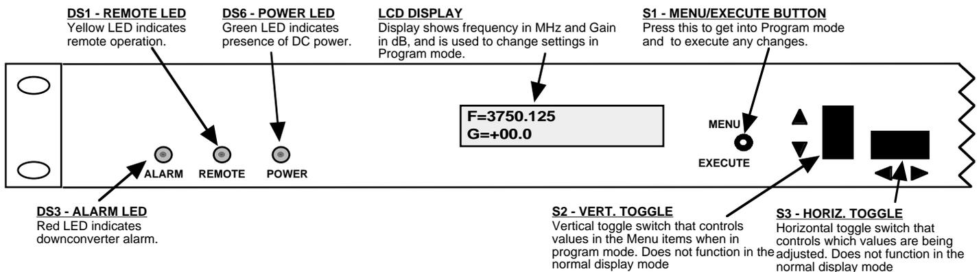
**FIGURE 2.3 2016-37 Front Panel Controls and Indicators**
