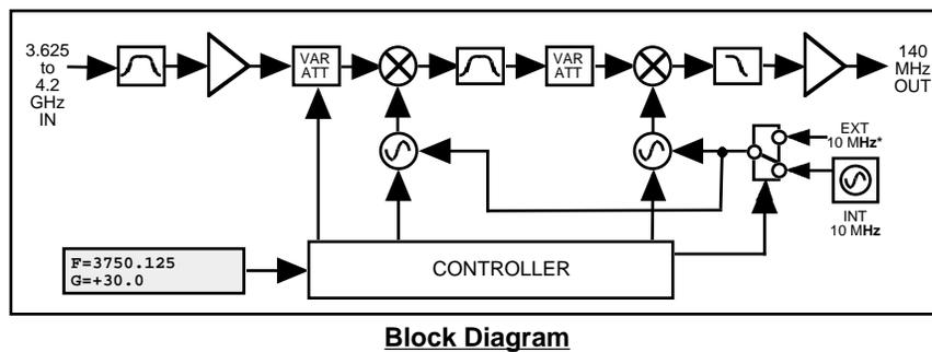
**FIGURE 1.2 Model 2016-37-140 Downconverter Block Diagram**
