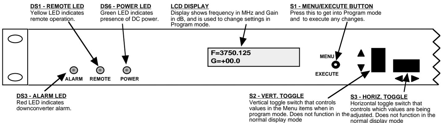
**FIGURE 2.3 2016-37-140 Front Panel Controls and Indicators**
