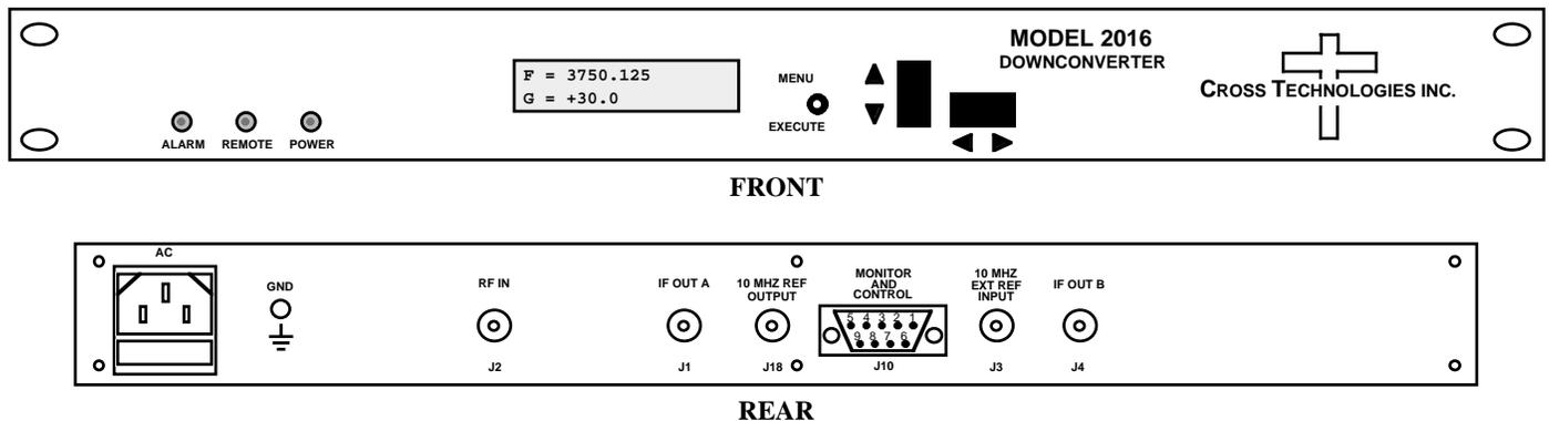
**FIGURE 1.1 Model 2016-37-140 Front and Rear Panels**
