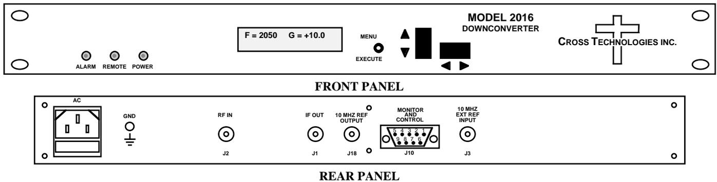
**FIGURE 1.1 Model 2016-26 Front and Rear Panels**
