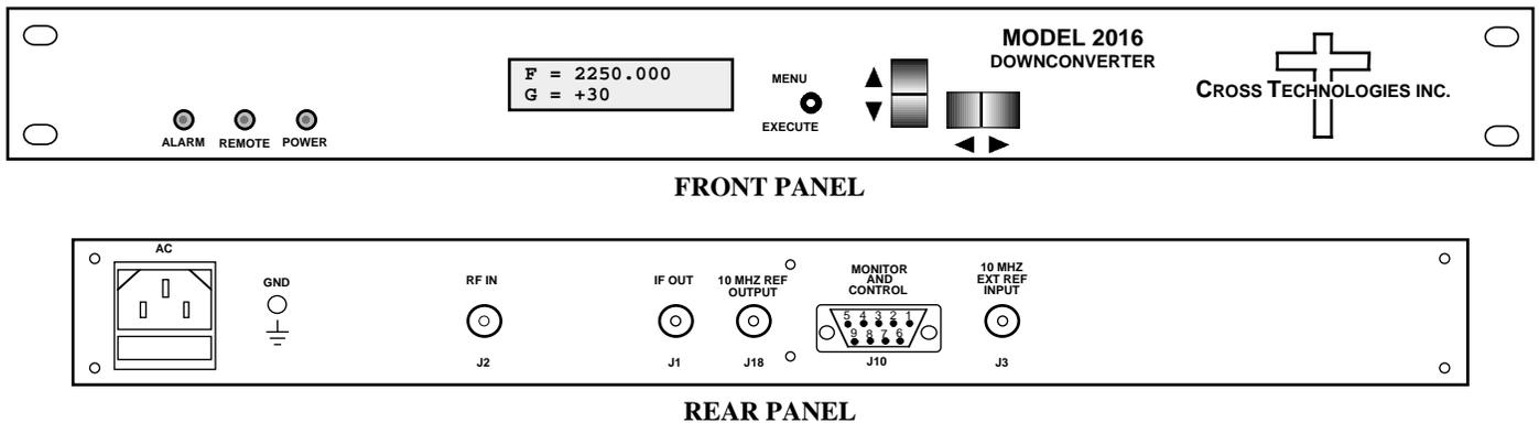
**FIGURE 1.1 Model 2016-2026 Front and Rear Panels**
