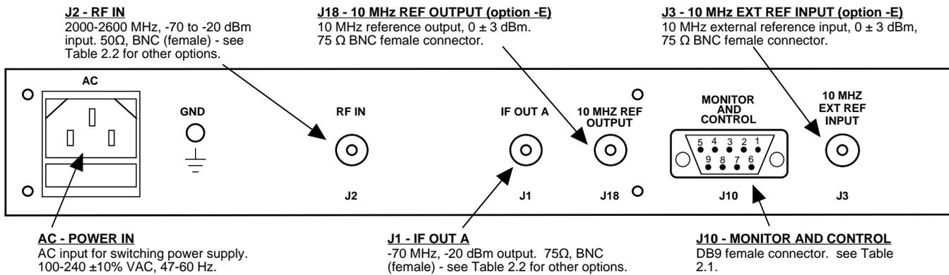
**FIGURE 2.2 2016-2026 Downconverter Rear Panel Inputs/Outputs**
